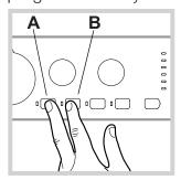
To start the programme press buttons **A** and **B** simultaneously for 5 seconds (see figure). The programme will start automatically and will run for about 70 minutes. To stop the cycle press the START/PAUSE button.
